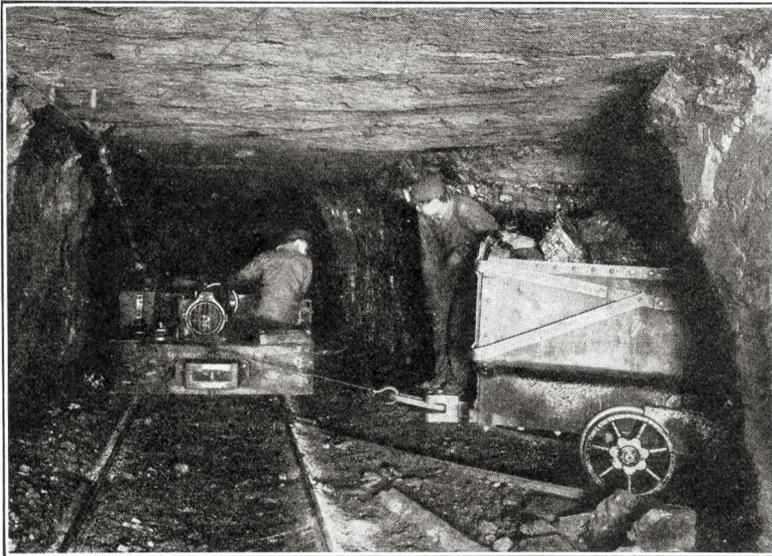
CONVEYING COAL IN A MINE BY ELECTRIC-MOTOR
